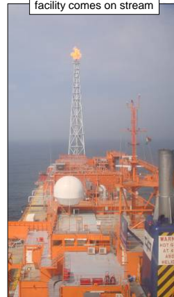
Gas flare marks first oil on Dhirubhai 1. Flare will be closed later this year when gas treatment facility comes on stream
